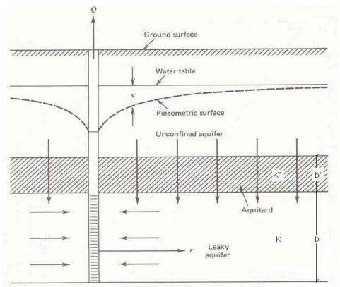
Figure 6.18 Well pumping from a leaky aquifer
