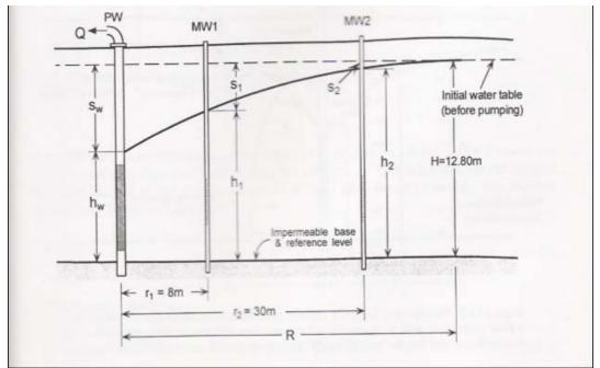
Figure 6.2 Pumping well with observation wells in unconfined aquifer
