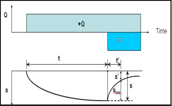
Figure 6.25 illustration of recovery test
