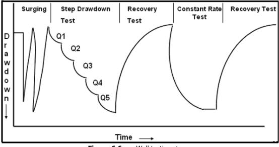
Figure 6.6Well testing stages
