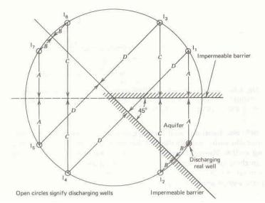
**Figure 6.37** Image well system for a discharge well in an aquifer bounded by two impermeable barriers intersecting at an angle of 45 degrees
