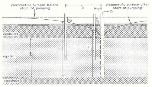
Figure 6.8 Cross-section of a pumped confined aquifer
