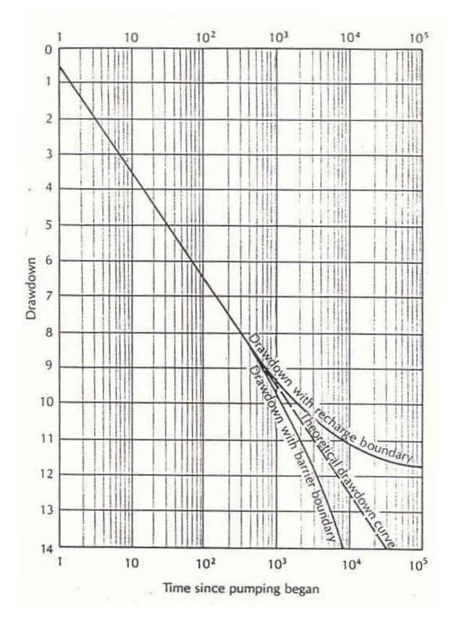
Figure 6.30 Impact or recharge and barrier boundaries on semi-logarithmic drawdown-time curve
