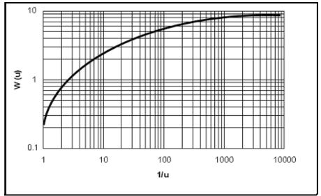
Figure 6.12 The non-equilibrium reverse type curve (Theis curve) for a fully confined aquifer
