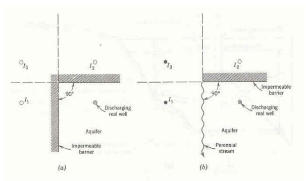
**Figure 6.31** Image well systems for a discharging well near aquifer boundaries. (a) aquifer bounded by two impermeable barriers intersecting at a right angles.(b) Aquifer bounded by an impermeable barrier intersected at right angles by a perennial stream. Open circles are discharging image wells; filled circles are recharging image wells.
