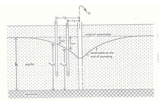
**Figure 6.9** Cross-section of a pumped unconfined aquifer (steady-state flow)
