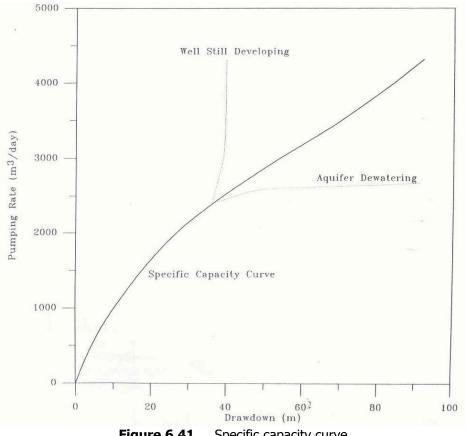
Figure 6.41 Specific capacity curve
