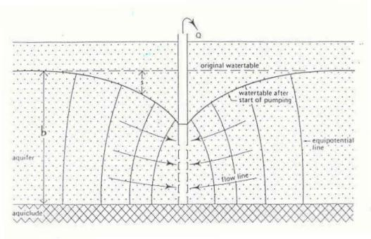
Figure 6.10 Cross-section of a pumped unconfined aquifer
