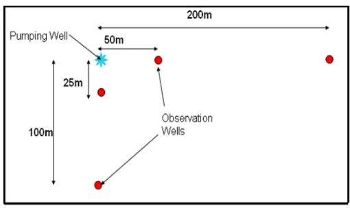
Figure 6.7 Borehole array for a test well
