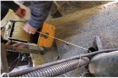
Figure 6.5 Measuring water level by M-scope
