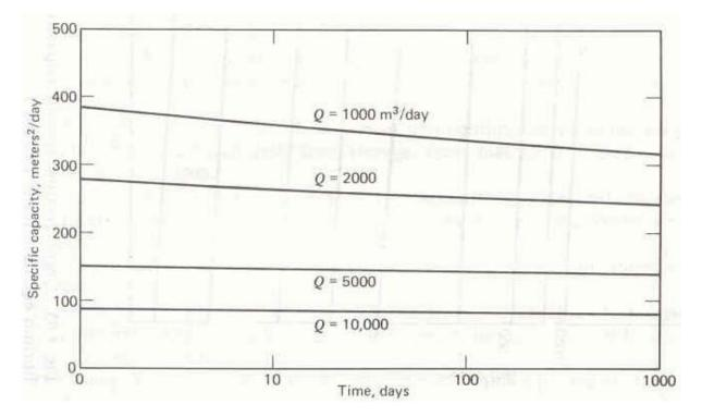
Figure 6.39 Variation in specific capacity of a pumping well with discharge and time
