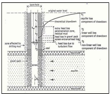
Figure 6.42 Variable head losses in a pumped well
