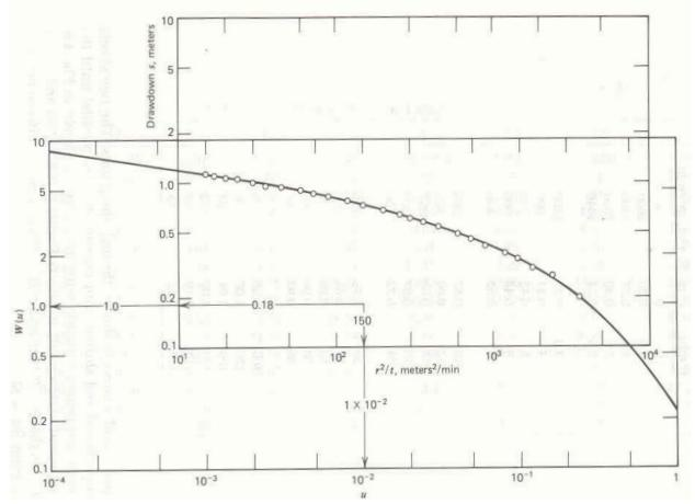
Figure 6.53 Theis method of superposition for solution of the nonequilibrium equation
