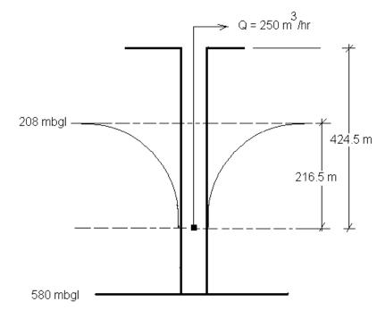
$$P = \frac{\rho \, g \, Q \, H}{746 \, \eta} = \frac{1000 \times 9.81 \times 250 \times 424.5}{746 \times 0.7 \times 60 \times 60} = 554 \ hp > 400 \ hp \ (the \ current \ pump)$$
