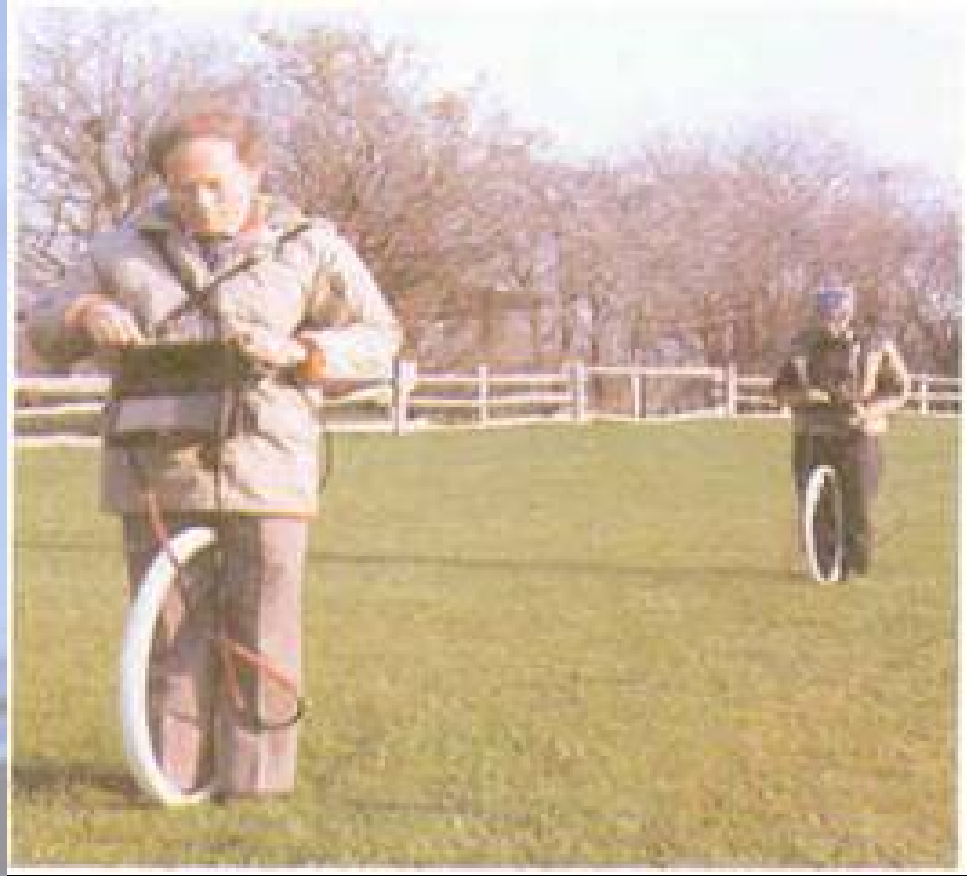
Figure 4.17: Hand-carried terrain conductivity devices use electromagnetic waves to measure the conductivity of earth materials. Direct contact with the ground is not required during data gathering. Thus, subsurface information can be obtained quickly in both highly urbanized and rural environments.
