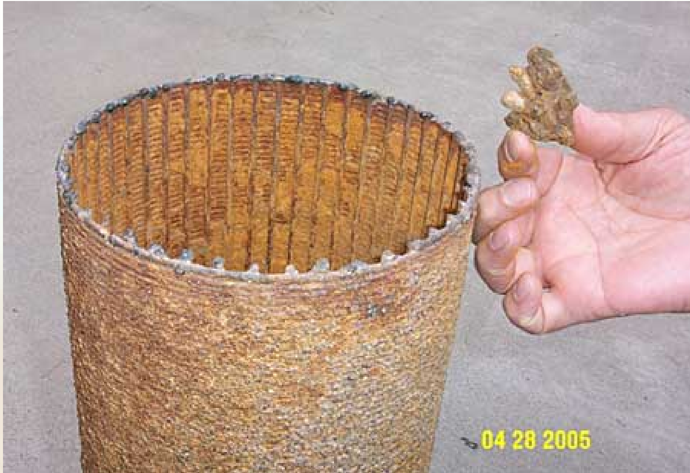
Figure 4: incrustated and plugged well screen along with an example of cemented gravel from the aquifer materials outside the screen
