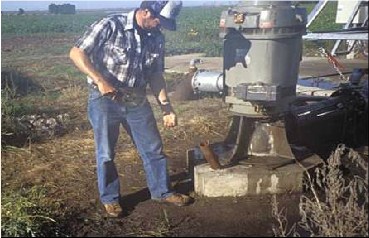
Figure 2.1: Measuring the water level in a well with a steel tape.
