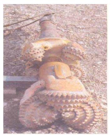
Figure 5.2: Roller or cone-type bits are preferred when drilling consolidated rock.
