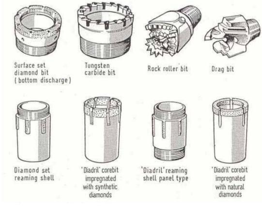
Figure 5.3: Different types of bits
